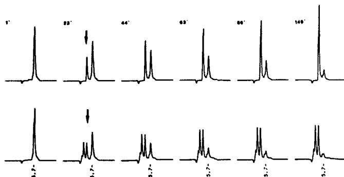
Figure 2. HPLC of NHS-BAT ester 1 in presence (lower) and absence of lysine (upper panel) at pH 8.3 as a function of reaction time; Arrows indicate the appearance of the side product.
